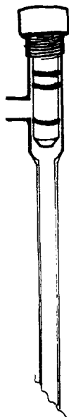
Figure 1. Teflon lined NMR tube with Teflon valve. The lining extends above the "O" ring seal but not into the side arm.
